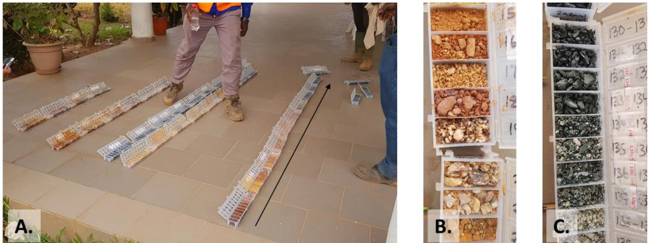
*RC Chip tray from the 2019 first pass drilling campaign. A. Three RC holes grading from surface to depth and transitioning through the weathered zone into the fresh rock at around 50m. B. High grade, weathered mineralised section of quartz-vein and host rock. C. High grade zone within host rock.*
